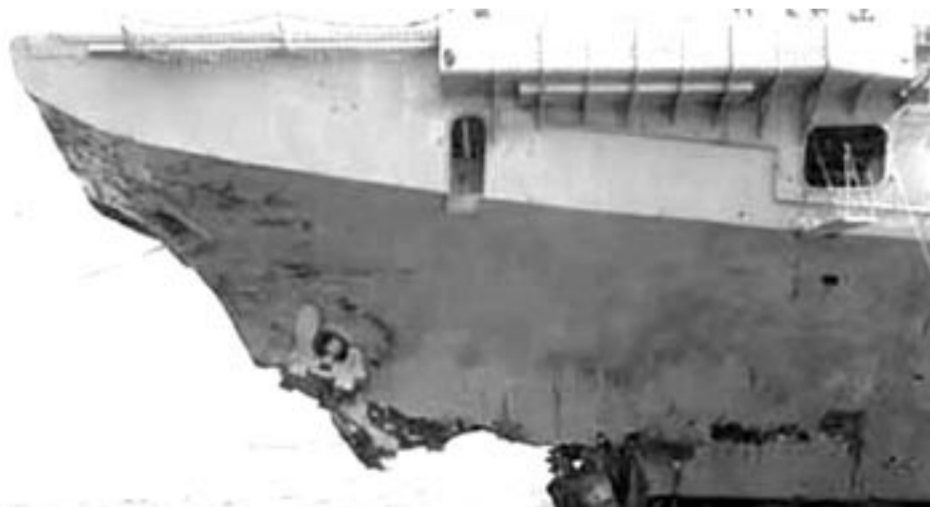
Part of the damaged bow of HMAS Melbourne after the collision with Voyager.
